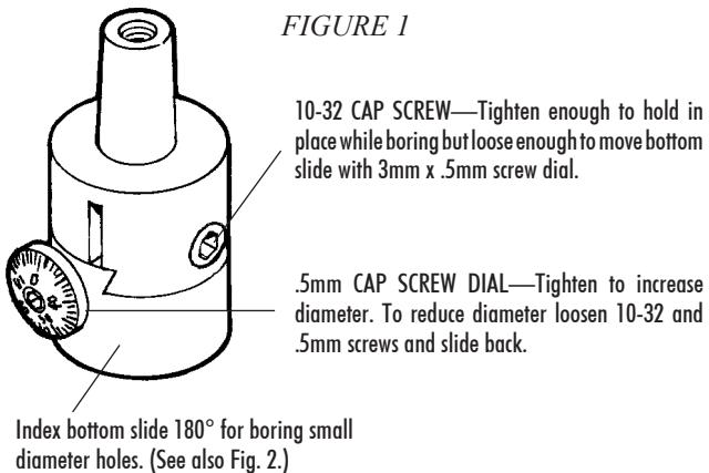
Tools put in the Sherline boring head should be as short as possible to keep setups as rigid as possible. It is easier to bore a hole completely through a part than to cut into a flat bottom hole. The problem is tool chatter when you get to the bottom. A hole has to be started with a drill to the full depth of the finished hole. Many times the work will require a special boring tool that usually can be made from a standard boring tool.
