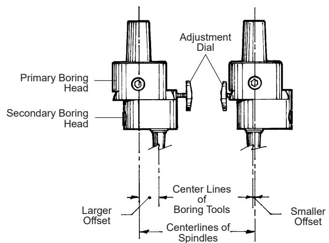
Clamp the boring tool into the boring head so the cutting face of the tool is in alignment with the center of the spindle. Adjust the tool in or out to take approximately .5mm cut in aluminum.
