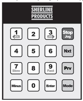
Figure 2—Layout of the keypad.
