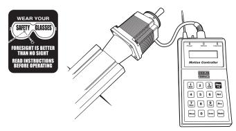
**NOTE:** The controller power supply is 110-240VAC compatible. It automatically switches from 110V to 240V for countries with 220-240 volt electrical current. The original power supply that we offered with this product was 110 VAC only.
