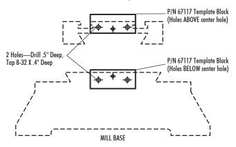
FIGURE 1—The rectangular block is used for the mill table and base. On the table, the two new drilled holes are ABOVE the existing center hole. On the base, the two new holes go BELOW the center hole as shown in the drawings above.
