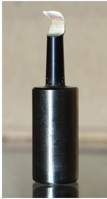
FIGURE 7—The tip of the P/N T3061 boring tool is shaped to undercut the final bore diameter to release the inner cubes.
