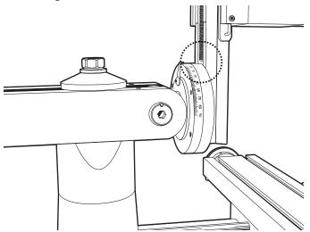
FIGURE 6—Notice the gap between the bottom of the leadscrew and the top of the movable clamping disk, highlighted by the dashed circle.
