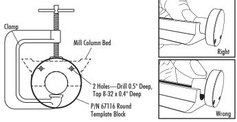
FIGURE 2—The round center of the template block registers in the center portion of the mill column bed, not on top. Rotate the template until the holes are level and clamp in place while starting holes.
