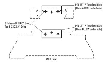
FIGURE 1—The rectangular block is used for the mill table as well as the mill base. On the table, the two new drilled holes are **ABOVE** the existing center hole, while on the mill base, the two new holes go **BELOW** the center hole as shown in the drawings above. **NOTE:** Mills made after 2002 may already have these holes in place.
