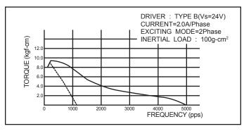
FIGURE 1—Motor torque curve
