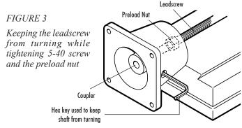
NOTE: The hex key adjustment hole may be located on either side depending on the axis. On older models the hole may be on the bottom instead of the side as is shown here.
