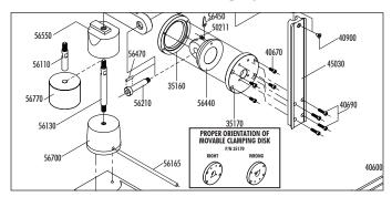
FIGURE 5—Shows the proper orientation of P/N 35170.
