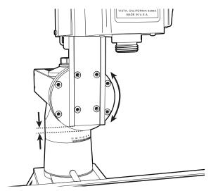
FIGURE 7—Notice the space between the bottom of the column bed and the bottom of the movable clamping disk, highlighted by the dashed lines.
