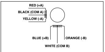
FIGURE 2— Color of internal wiring for NMB motors
