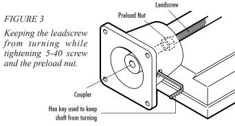
NOTE: In the drawing above, the mill base is used as an example, but the same technique is used on the lathe. The hex key adjustment hole may be located on either side depending on the axis. On older models the hole may be on the bottom instead of the side as is shown here.
