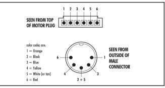
FIGURE 3: diagram shows which pin in the DIN connector is wired to which position in the motor connector.
