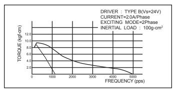
FIGURE 1—Motor torque curve
