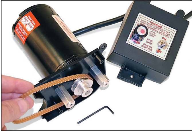
FIGURE 3—Place belt over motor pulley.
