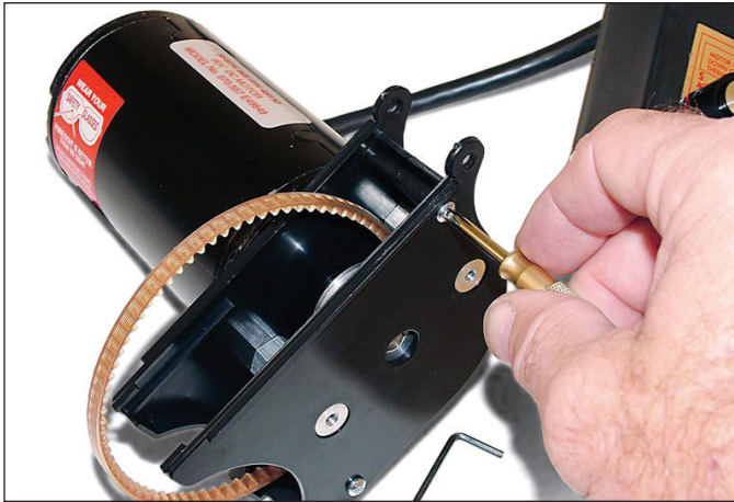
FIGURE 4—Attach outer belt guard.
