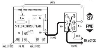
FIGURE 1—Wiring the switch to reverse motor direction. Also shown are lug attachment points and wire colors for the Sherline DC motor.
