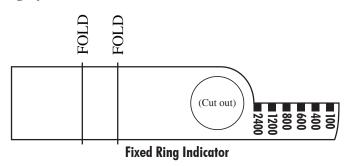
The above indicator can be used if desired to help you tell which ring is which when the gauge is moving. The hole slips over the spindle and the end is taped to the speed control housing. It's a bit crude, but some might find it helpful.
