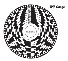
Make a photocopy of the above gauge, cut it out and glue it to the Sherline spindle pulley. Use under 60 Hz fluorescent light for best results.
