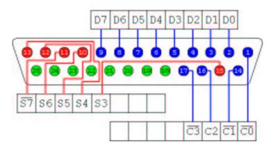
Diagram of the 25 pin connector used on most computers for connecting to the printer. Refer to the following subsection for pin assignments when using EMC.
