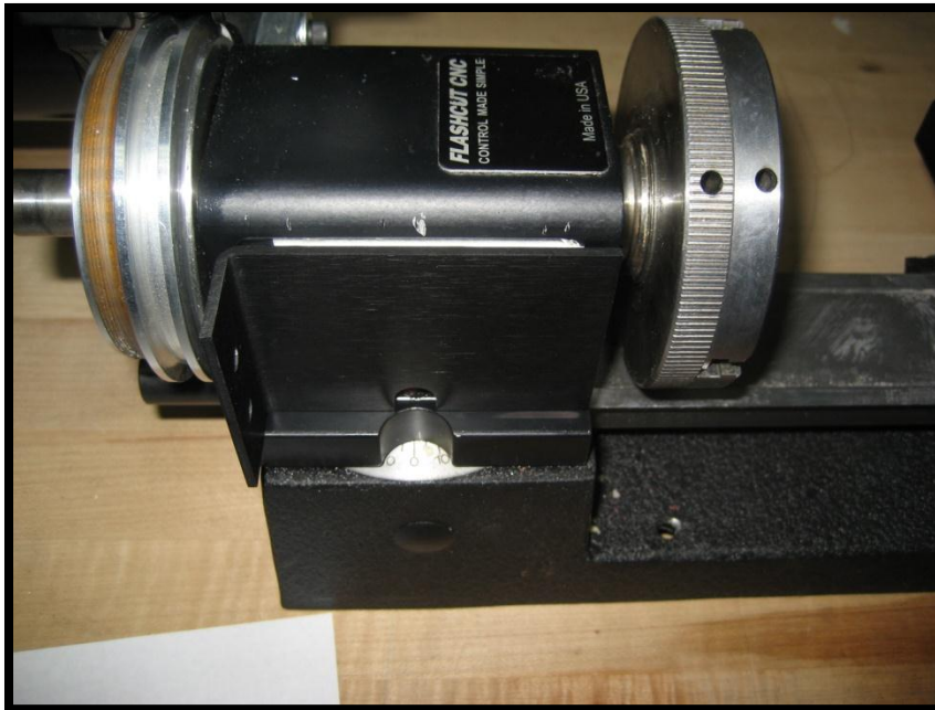
Figure 4. Small Encoder Bracket attached to spindle assembly with double sided tape.
