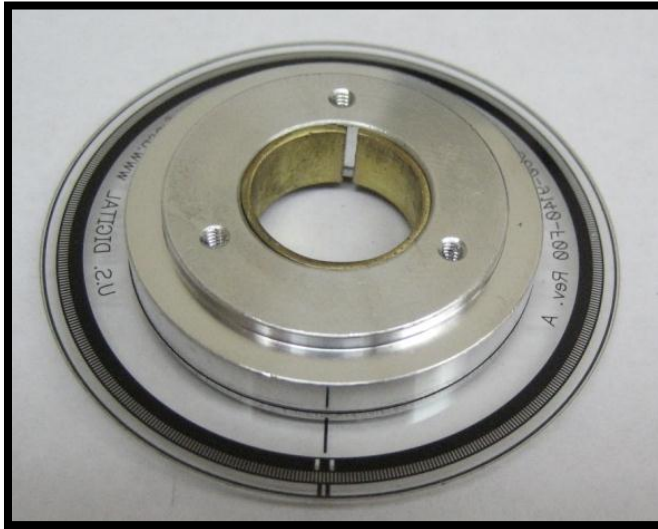
Figure 7. Brass ring seated into encoder hub.
