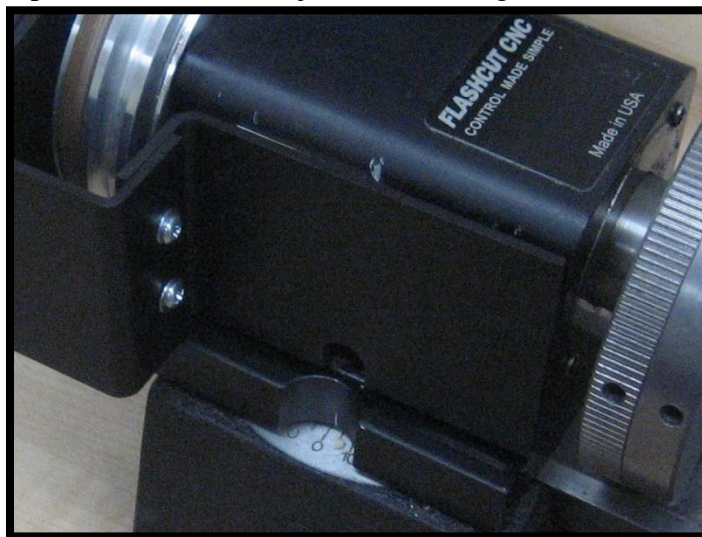
Figure 6. Small Encoder Bracket attached to Large Encoder Bracket.
