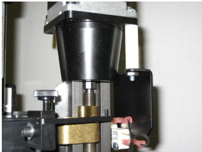
Figure 9. Z+ Limit Switch inside view.
