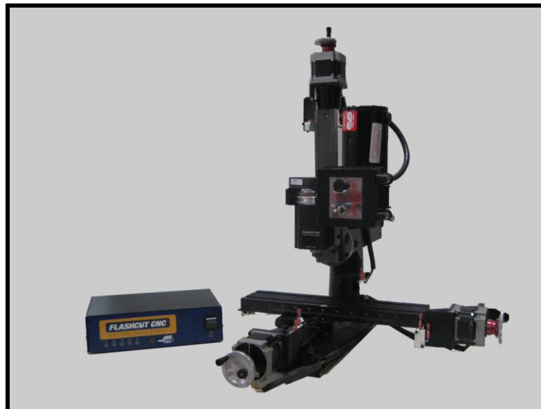
Figure 2. FlashCut CNC 2000 CNC mill with Limit Switch Kit installed.
