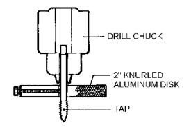
The tap is held in perfect alignment by the chuck. When the chuck is loosened slightly, the tap can be rotated using the disk and your fingers which provides an excellent "feel" for the process. The tap goes in straight and is unlikely to break.
