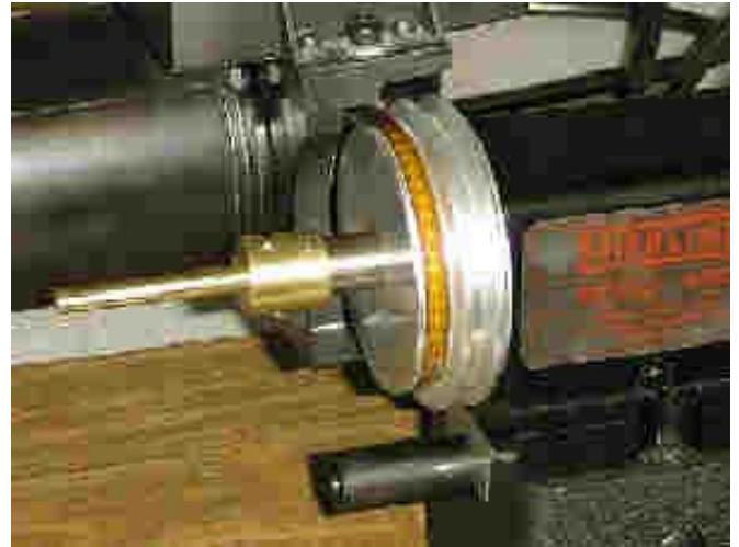
Figure 2—This photo shows how the depth rod is attached to the lathe spindle. Loosening the outer set screw allows you to adjust the rod for depth.
