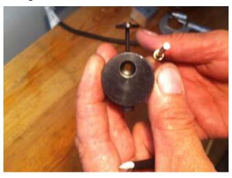
After separating the Boring Head secondary (bottom), and retracting the Adjustment dial Screw, use a Tommy Bar as a puncher to push the Boring Tool out.
