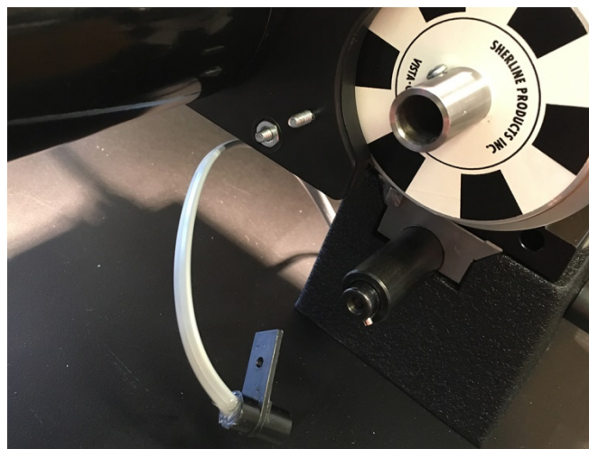
Figure 3 — Now, I have a #6-32 post where I can secure the tach sensor with a knurled thumb nut.
