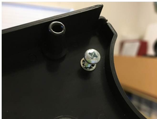
Figure 2 — Then installed a #6-32 x \frac{3}{8} " machine screw with an internal star lock washer.
