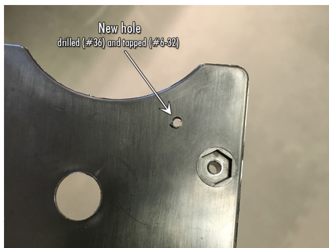
Figure 1 — I drilled (#36) and tapped (#6-32) the hole.
