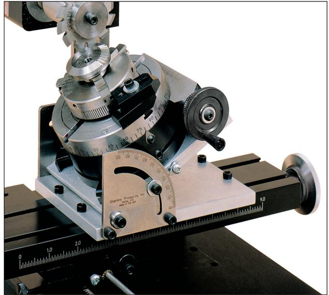
*FIGURE 3—A complex setup shows a part held in a 3-jaw chuck, which is mounted to the rotary table, which is mounted to the tilting angle table, which is in turn mounted to the mill table. A mill arbor holds a gear-tooth cutter which is cutting teeth in a bevel gear. The horizontal milling conversion is used to mount the headstock in the horizontal position. With Sherline tools and accessories, the parts you machine are limited only by size, not by complexity.*
