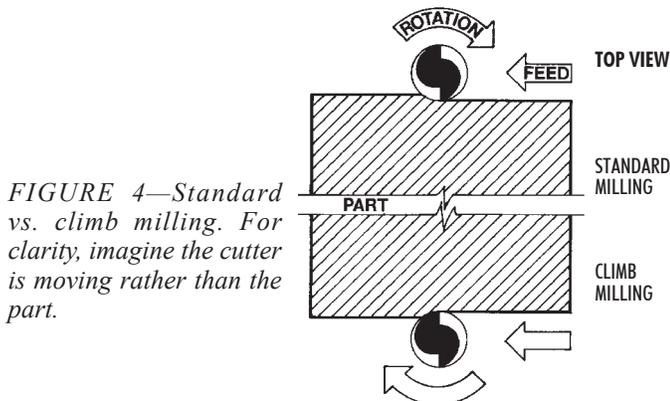
FIGURE 4—Standard vs. climb milling. For clarity, imagine the cutter is moving rather than the part.
