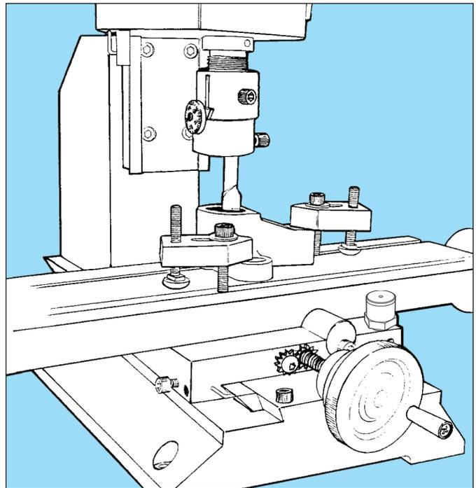
FIGURE 5—Boring the inside of a hole to exact size with a boring tool held in a boring head.
