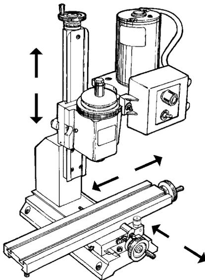
FIGURE 1—The axes of movement for milling on a standard 3-axis vertical milling machine.
