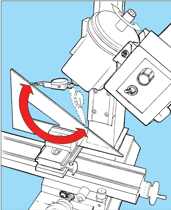
FIGURE 9—Indicating in a 30° head tilt using a mill vise and draftsman's triangle
