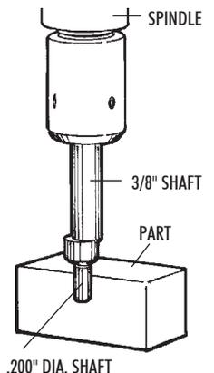
FIGURE 8—Using an “edge finder” to accurately locate the edge of a part.
