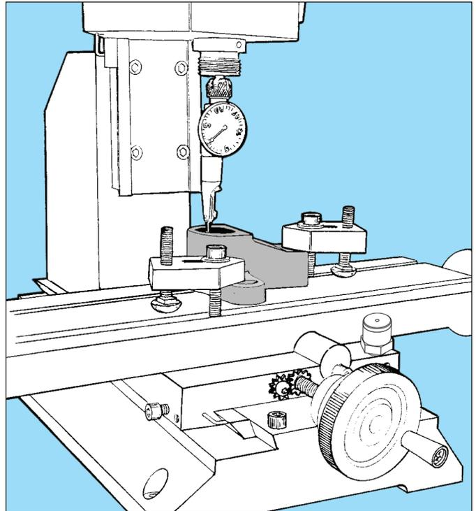
FIGURE 7—Indicating in the center of a hole.
