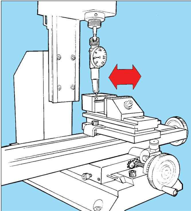
FIGURE 6—Indicating in the jaws of a vise. Shown is a Starrett “Last Word” Indicator. Starrett gauges are available in numerous sizes and types. They are manufactured in Athol, Massachusetts and can be purchased from most industrial dealers.
