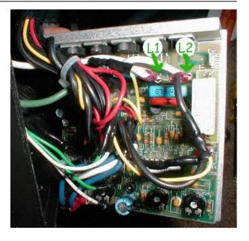
Connect the indicator lamp wires to terminals L1 and L2 on the Sherline speed control circuit board.
