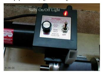
Adding an indicator light is very easy. Just buy a 110 volt indicator light from your local Radio Shack [electronics] store. They come in a number of colors but I chose red to get my attention and indicate a warning. Drill a hole in the plastic case and connect the wires directly to L1 and L2 on the PC board. That's it. Now when the lathe or mill is **ON** you will have a light to let you know. Quick, cheap, and most importantly, **SAFE**.
