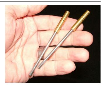
If you don't have a knurling attachment, you can simply turn grooves in the end for grip as Larry Simon did on these brass ends, which are pressed onto standard Sherline Tommy bars.
