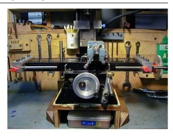
The left-hand photo shows the Y-axis depth stop. Here Tracy tried a knurled brass knob to lock the bar but felt it couldn't be tightened enough to keep the rod from moving. He now uses screws with a larger plastic handle for more leverage but suggests a small piece of brass between the end of the screw and the rod will protect the surface of the rod. In the right-hand photo both the Y-axis and X-axis locks can be seen.
