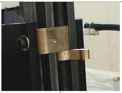
Tauseef says: I finally figured out a simple way to control backlash. First, drill and tap two holes, one in the saddle and one in the nut (length wise). The nut has to go on upside down for this setup. The indentation for the "ball" that fits in to lock the manual mill faces up. I also put the nut on the bottom of the saddle so it doesn't unscrew when the Z axis is at the top.
