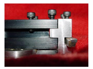
simple aluminum adapter that attaches where the tool would normally be and lowers it exactly 1/4". No drawing was provided, but you should be able to come up with dimensions yourself. It's pretty straightforward once you see how it works.
