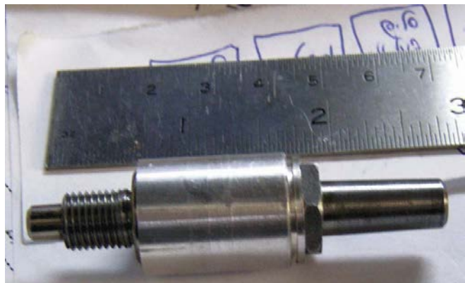
FIGURE 1—The bearing adapter is shown without the chuck attached. The Jacobs chuck screws onto the 3/8-24 thread. A Tommy bar hole in the body (not shown) allows the chuck to be tightened against the body.
