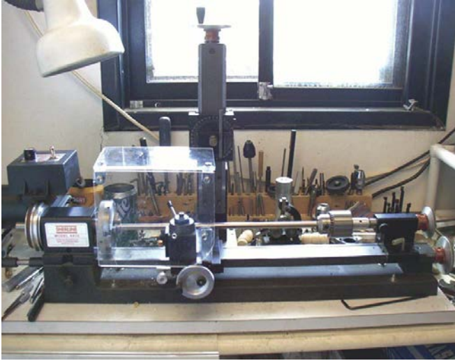
FIGURE 2—The lathe fitted with the live chuck adapter holds a long piece of stock. Behind the lathe you can see Dan's center-mounted milling column and some of his accessories. Notice also his custom chip guard.
