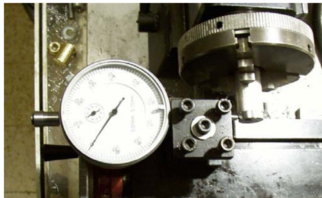
An indicator held in the round hole of the P/N 7600 3/8" tool post is held on the part's centerline.
