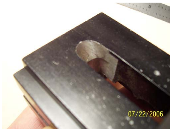
Photo 2—Seen from the top of the vise, a chamfered area allows the hold-down screw to extend farther back.
