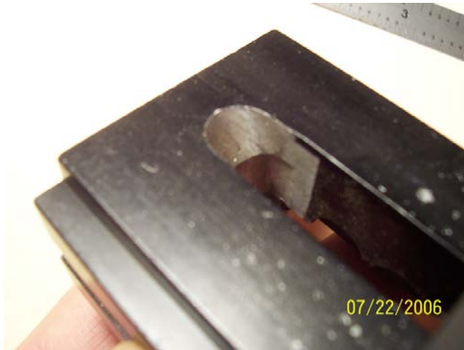
Photo 3—shows the new jaw opening to be as much as 2.5".
