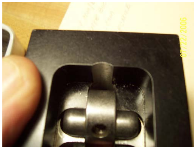
Photo 1—The back of the slot is extended as seen from the bottom of the vise.
