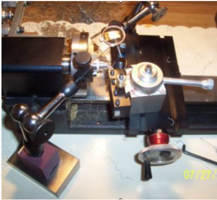
(Left) Dental mirror attached to block. (Middle) End of part in natural shop light. (Right) End of same part with light reflected on end of part by dental mirror. (Sorry, no larger image available for 3rd photo.)
