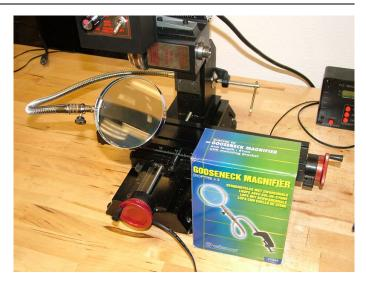
Only one photo is needed for this one, it's pretty selfexplanatory. The gooseneck clamp attaches to the mill base and the 3x magnifier allows you to see small work up close.
