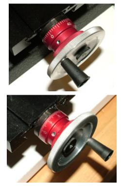
An inch handwheel (left) has 50 marks, each indicating .001" of actual table travel. A metric handwheel (right) has 100 marks. When used on an inch machine, each of the 100 marks now indicates .001" removed from the diameter of the part. Shown are adjustable zero handwheels.
