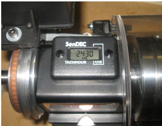
Photo 1—The readout unit is glued to the top of the headstock on the lathe. (On a mill it is glued near the pulley so it reads properly with the headstock held vertically.)
