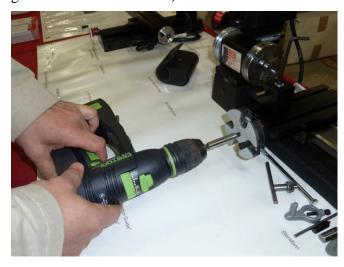
A reversible, battery powered electric drill makes quick work of long travels in either direction. An electric screwdriver would work too.
