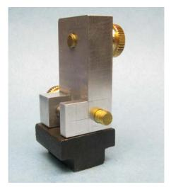
The first drawing shows the dimensions, while the other two show the finished parts. The knurled brass knobs on the attachment screws are a professional touch. They are bonded to the threaded brass rod using Locktite permanent liquid adhesive. The knobs are available for use on electrical contact posts if you don't want to make your own. Brass is used to keep from damaging the surfaces of the bed and table.
