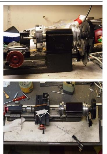
In these photos you can see how a right-handed operator might find this positioning of the lathe more comfortable to use. With the motor and speed control out of the way, there's no reason not to if you don't mind the unconventional positioning of the lathe.
