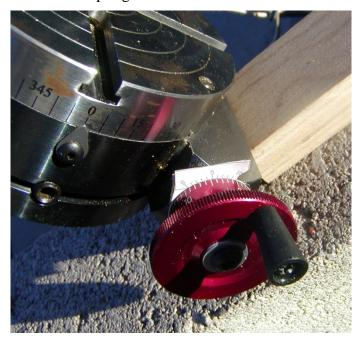
Here is the printed Vernier scale cut out, installed behind the handwheel and taped to the worm housing. The "10" mark on the scale lines up with the witness mark on the worm housing.
