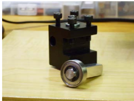
The holder uses a simple 3/8" shank in the P/N 7600 tool post. A skateboard bearing is attached to one end.
