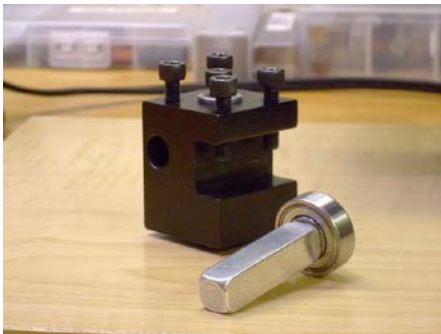
The holder uses a simple 3/8" shank in the P/N 7600 tool post. A skateboard bearing is attached to one end.
