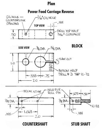
"Using the two 20-tooth, 24P gears (P/N 31200) from the P/N 3100 threading kit and adding a parallel countershaft to accommodate a gear, reversal is accomplished. As you can see from the photo, the countershaft is equipped with two roll pins for the gear motor coupling and to engage the gear. The gear motor simply sits on the same base as the lathe and is not fastened down. To reverse the carriage you just move it from one shaft to the other.
