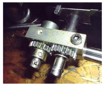
By powering the countershaft on the left the carriage is driven in the reverse direction. The main shaft on the right is extended to drive it in the standard direction. The power feed motor unit is not fastened down and can be moved to either shaft end depending on the direction desired. A store-purchased 3/8" collar with set screw fits on either end of the countershaft to hold the second gear in place and locate the shaft.
