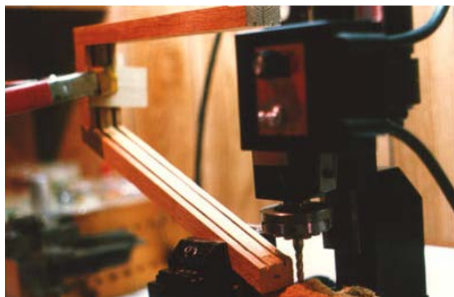
Machining the angles on the corner of the framework
