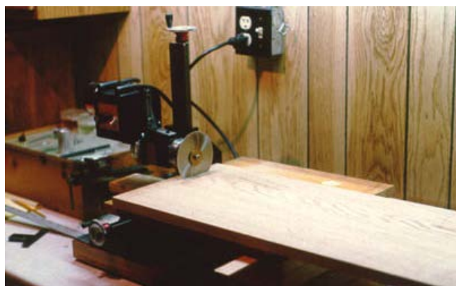
Cutting a 12" wide by 3/8" thick solid oak plank with a slitting saw
