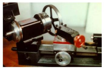
Finishing the outer edge and back edge of a large wheel. The headstock is lifted using a riser block to get an additional 1.25" clearance. By turning the headstock at a  $45^{\circ}$  angle and using the compound slide at a  $45^{\circ}$  angle with a cutting tool also angled at  $45^{\circ}$ , Pam was able to finish the outside and back faces.
