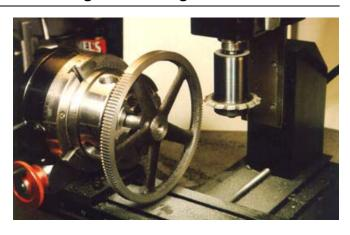
The gear teeth are being cut into the wheel using an involute gear cutter on a long arbor. The wheel just clears the table using the standard vertical rotary table setup. A chuck mounted to the rotary table holds an arbor that secures the wheel by its center hole. The small closeup (previos photo) shows the nice tooth form.
