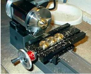
These two photos show Keith's setup to turn the taper and Oring grooves on the train's wheels.
