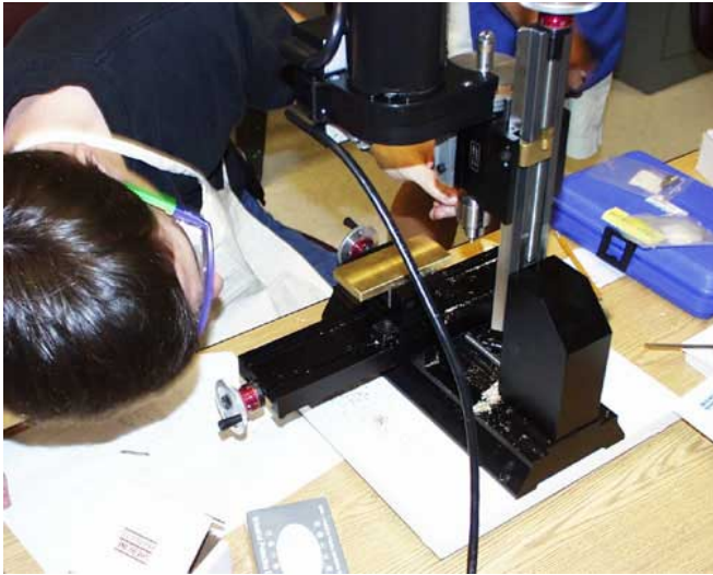
A student inspects his work as a precision gauge block emerges from a chunk of brass.
