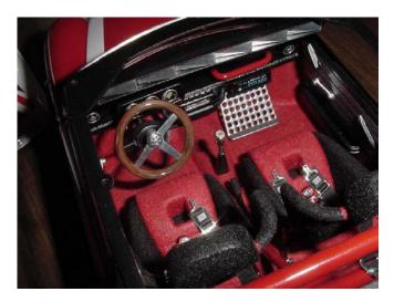
With the roof removed, interior detail can be seen. The steering wheel is machined from aluminum like the one on the Lotus above. The wood grain effect is achieved with paint. The kick plate on the passenger side floor was to help the passenger brace himself into his seat during "spirited" handling. The kit is offered only in right-hand drive, so Mark converted this one himself to left-hand drive for those of us in America who drive on the "wrong" side of the road.
