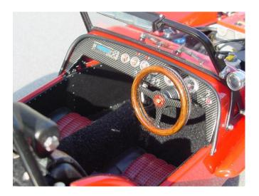
The interior features a carbon fiber dash inset with detailed instruments turned up from aluminum. The steering wheel was also custom made from aluminum. The wood grain look is achieved with paint.
