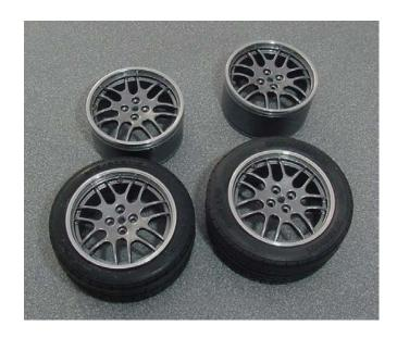
Mark is now working on a seventh model of the Lotus 7. It will include more detail and custom made metal parts than any car he has made in the past. In honor of the seventh seven, notice the custom seven-spoke aluminum wheels he has machined. They include valve stems with separate cores that move within the stem just like the real thing.
