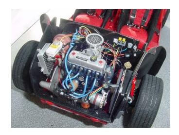
With the front end of the car removed, details of the 1300 cc fuel-injected engine can be seen. (This owner has boosted this already potent package with the addition of an aftermarket Nitrous Oxide system.) The Mini was the first car to place the engine sideways and use front wheel drive in order to maximize interior space; the layout now used in most modern cars. If you like old Mini's, buy or rent an old movie called "The Italian Job" starring Michael Caine. The cars are the real stars.
