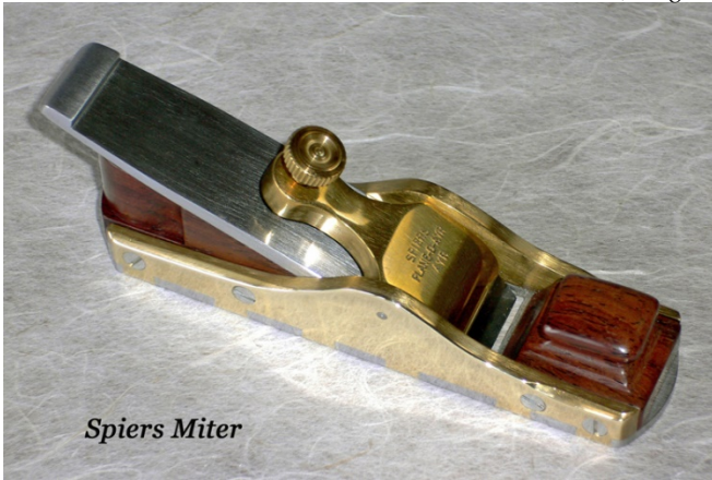
A Spiers miter plane with dovetailed sole plate.
