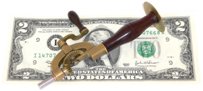
A French Drill with beveled gears and hand crank. A plate at the end of the handle allowed the user to lean his chest on the drill to apply extra pressure to make the cut go quicker.
