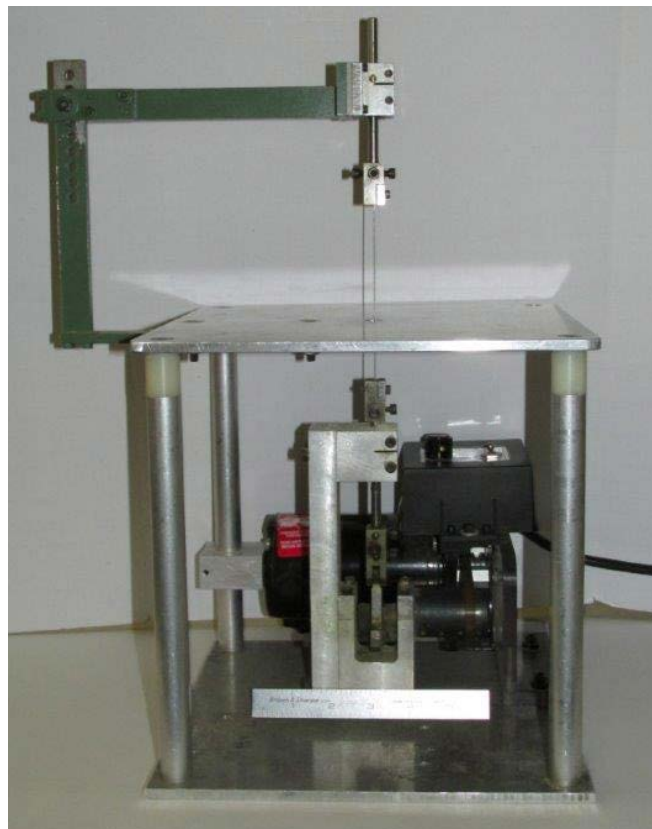
Photos 1 and 2—The finished scroll saw is seen from each side.
