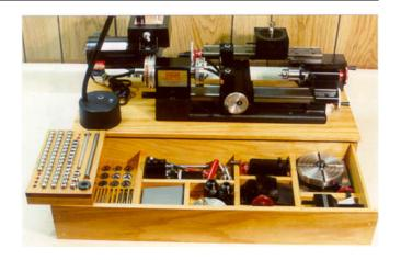
Just add electricity and you're in business virtually anywhere. A drawer underneath includes all the accessories. The vertical milling column is mounted behind the lathe for travel. A high intensity light with a flexible arm is mounted at the left corner.
