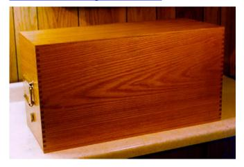
Notice the finger joints at each corner on the cover. The case is 26" long by 11" wide by 13" high and made from 3/8" oak.
