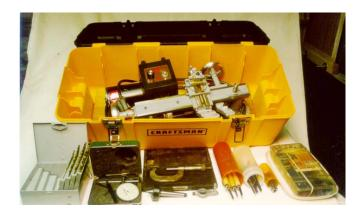
The wooden base with partially disassembled lathe is set in the tool box. Other components like a drill index, measuring tools and accessories are fitted into the compartments around the sides.
