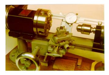
Here the carriage is fitted with a compound slide. In the back you can see the dial caliper mounted to indicate carriage position.
