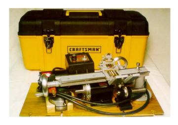
The lathe comes apart and the tailstock and motor/speed control unit are mounted to the base. The chuck also has a fitted compartment.
