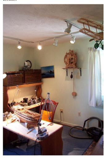
About the clocks, Chris says, "I cut the gears using the milling column with the rotary table and a slitting saw. The shafts were all turned down on the lathe. Turned out nicely, and keeps good time. Everything but the clock dial and hands are Beech, the hands are walnut with a cherry plywood dial
