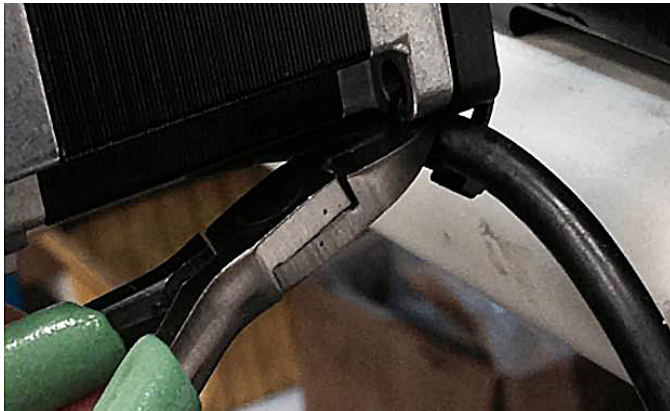
FIGURE 2—Carefully snip the zip tie so you don't cut into the motor cable.
