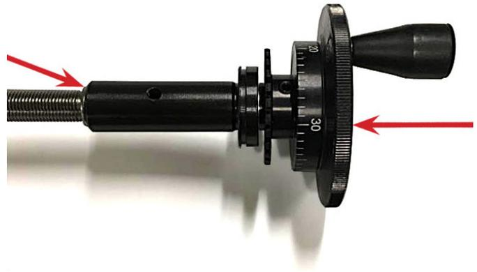
FIGURE 4—Red arrows show the shoulder on the leadscrew and the force point on the handwheel to sandwich the washers
