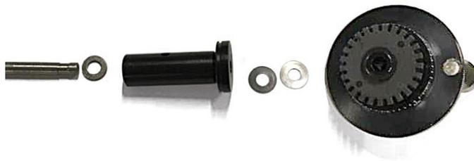
FIGURE 1—From left to right: Leadscrew, 1/4" washer, DRO Leadscrew Thrust, two shim washers, DRO handwheel.
