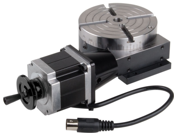
FIGURE 23—The Sherline 8730 CNC Rotary Table with stepper motor can be plugged directly into the A-Axis cord pre-wired into your computer to operate as a 4th axis.
