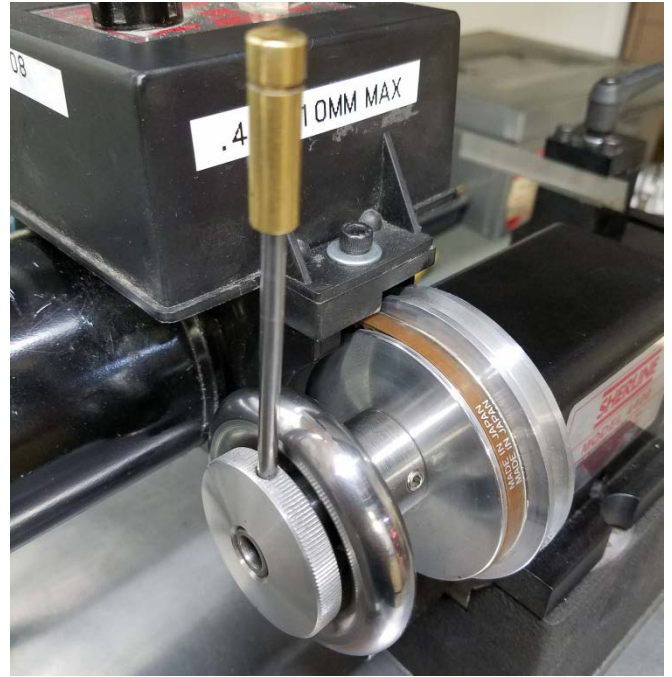
Figure 3—Tommy bar inserted into the new #21 hole.
