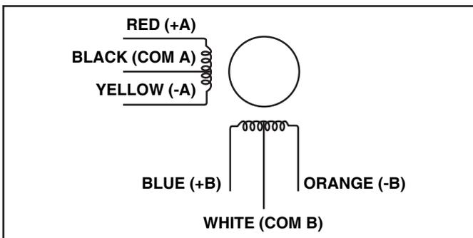
FIGURE 2— Color of internal wiring for stepper motors
